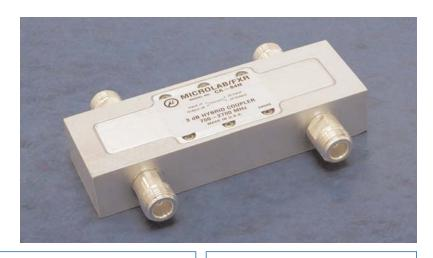
Microlab Model CA-H70, is based on catalog model CA-84N. This 4 port Hybrid Coupler is designed to meet the special needs of the wireless market, commonly being used to combine two wireless carriers with powers up to 80W, in the band to a single antenna feed. Isolation is maximized while passive intermodulation (PIM) is minimized.
